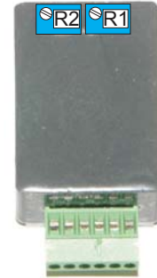
LOCATION OF CALIBRATION TRIM POTS, TOP VIEW
