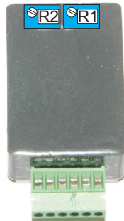
LOCATION OF CALIBRATION TRIM POTS, TOP VIEW
